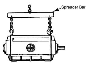
Typical Construction with Four Lifting Lugs
